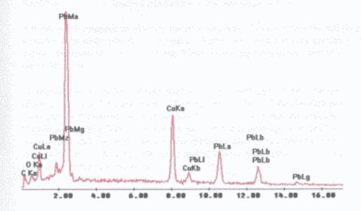
The overall analysis shows all the different peaks of Pb and Cu on the screen as well as some C and O... for which the operator did not really care or worry.
