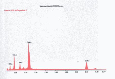
Depending on the exact positioning of the beam the relative Al peak becomes higher or lower.
