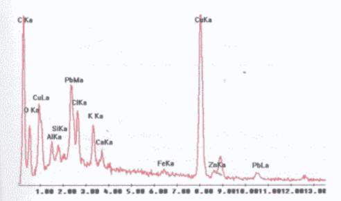
Without any doubt besides Cu and Pb (evident), there is undoubtedly the presence of C, O, Al, Si, K, Ca, Fe, Zn... Repeated verification with the operator proved the same conclusion. The elements are there in macroscopically quantities so that they cannot be attributed to the presence of impurities in the detection screen.
