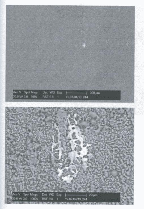
Visual inspection shows that the spot is also lead, but containing also heavier elements in it. It is created at the moment of the shot and is morphologically melted into the redistributed target material on the Cu screen.
