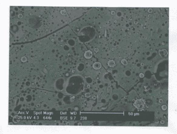
The backscattered pictures of sample 238 show the cracks in the aluminium surface. You can clearly see the splashes on the surface which, by morphology are a proof that the splashes are created and deposited "after" the shot but yet the splashes show that the material was still in a liquid form at the moment that it fell on the surface.
