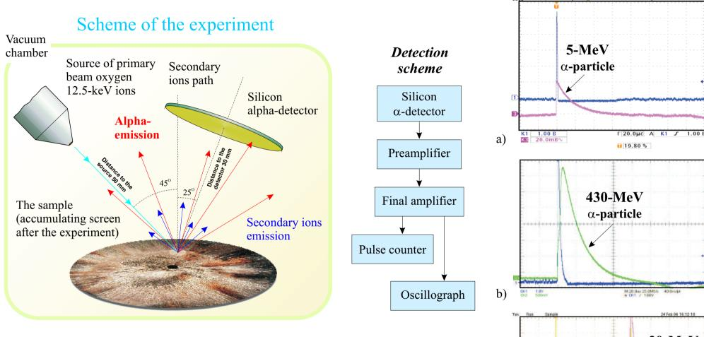
Background  $\alpha$ -particle pulse registered by  $\alpha$ -detector after 1.5 hours since the start of detecting with turned-off primary ion beam (a); pulse registered by  $\alpha$ -detector while studying the sample No. 53 (b); multiple pulse series registered by  $\alpha$ -detector while studying the sample No. 73 (c).
