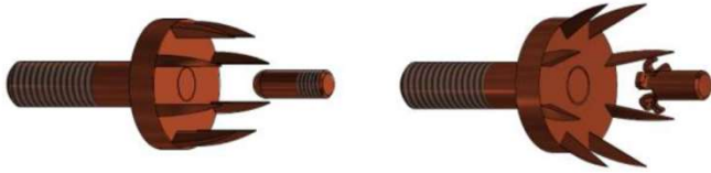
Fig. 12. Sketches of cathode - anode system before explosion (left) and after explosion (right). The cathode-anode system as part of the unit is shown in the sketch, see Fig. 4.
